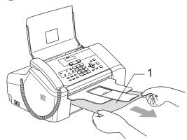
■ If you cannot remove the jammed paper from the front side, or the error message still appears on the LCD after you remove the jammed paper, please go to the next step.
